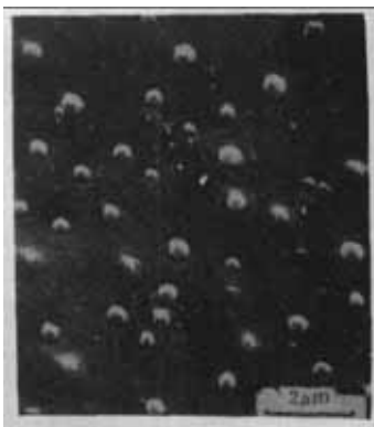
Fig.5 Fracture surface of PSF ( M_n = 18700 , 10phr) modified E51/Pip epoxy (Type A)
