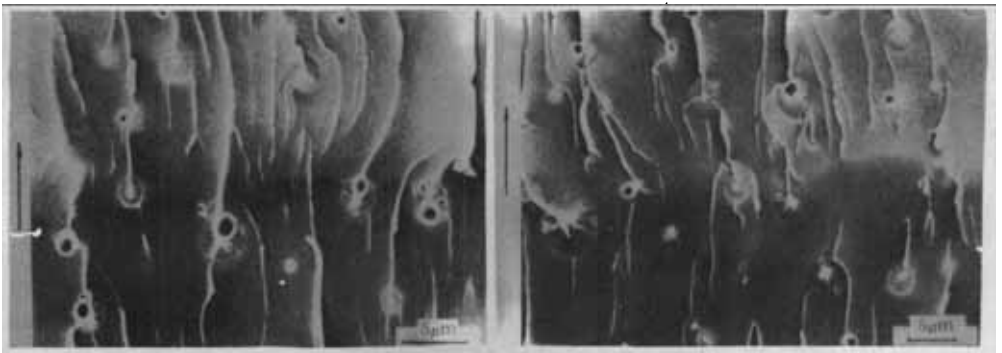
Fig. 13 and 14 The SEM fracture surface of PSF modified AG80/DDS epoxy (Direct evidence of the bowing out of crack front between PSF particles) These pictures were taken near the initial crack propagating line.
